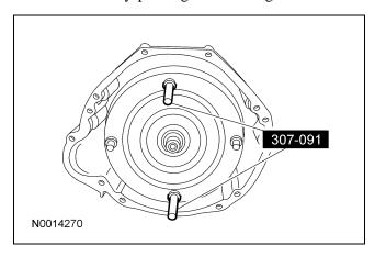
116. Lubricate the torque converter pilot hub with multi-purpose grease.
